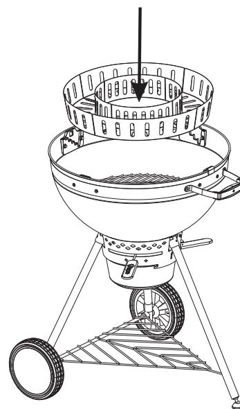
**11. Place the BBQ grate (5) with the BBQ grate handles (6) on the functional part (17).**
