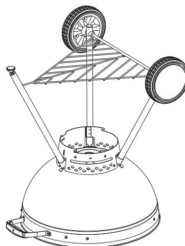
8. Attach the handle for the ash collecting cup (21) to the ash collecting cup (22). To attach it to the holder (20), hook it in sideways first and then let the front tab latch on.
