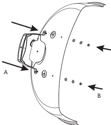
**13. Attach the thermometer (2) to the lid (3). Attach the parts to the inside of the cover in the following order: washer, snap ring, thumbscrew.**
