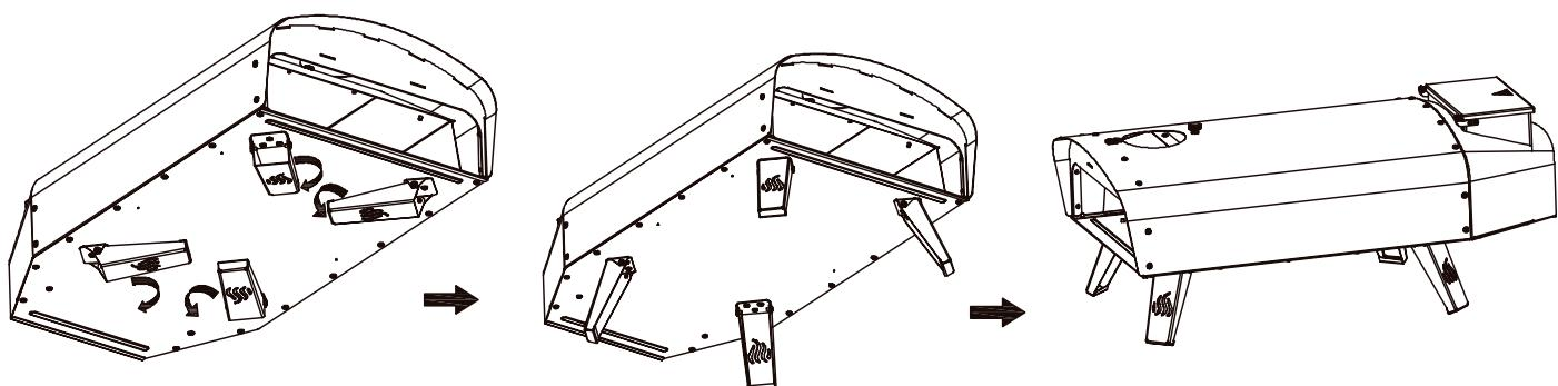
Fold out the four legs completely and place the pellet pizza oven on a flat, heat-resistant surface. Make sure you have a secure footing! Avoid a surface that can be easily scratched.
