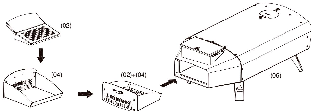
Place the pellet chamber (2) in the ash collecting tray (4).
