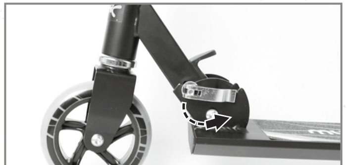
After you have folded out the handlebar stem upwards, the axle of the quick release locking system has to lock-in into the mount and the quick release lever has to be securely closed. If necessary, you can adjust the quick release locking system to the correct tension, by tightening or loosening the securing nut.
