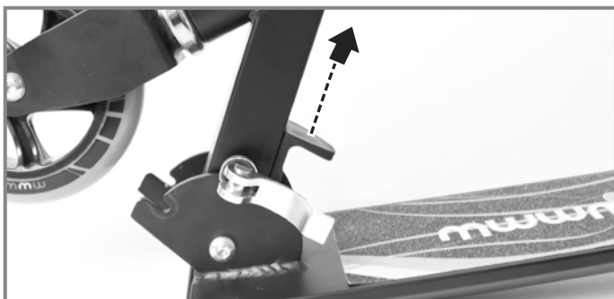
Pull the plastic handle upwards until the axle of the quick release locking system is released from the mount.
