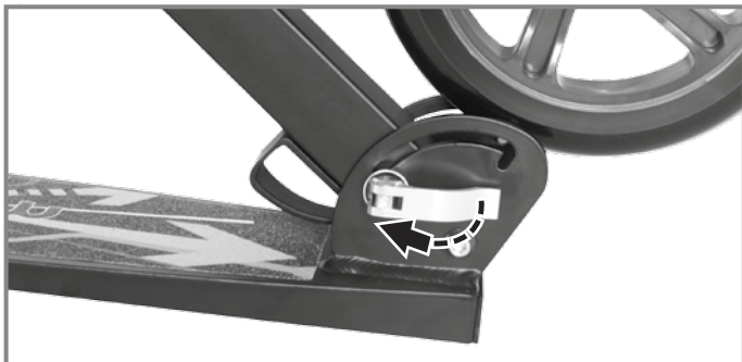
Open the quick-release lever.
