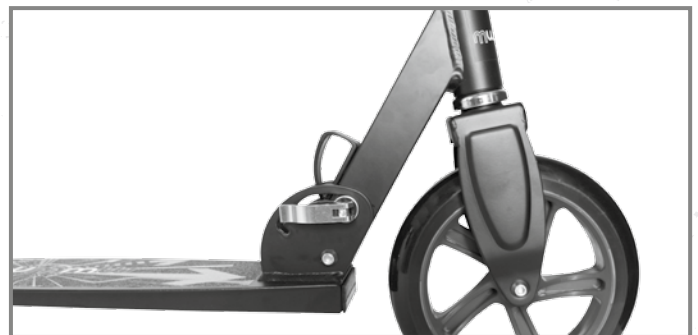
Folding-out the handlebar stem.
